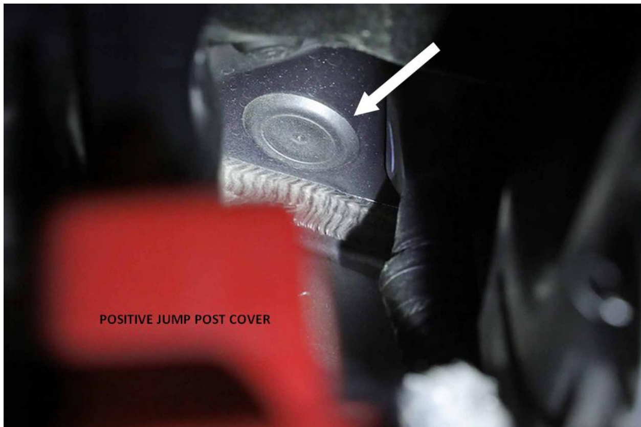
Figure 15: Pass Through Grommet (view from above in engine compartment, looking down in area behind the positive jump start post)
