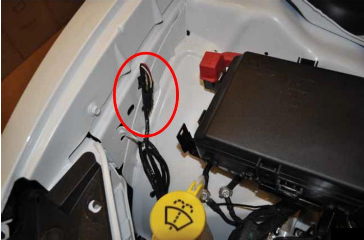
Figure 9: 12-way underhood pass-thru circuits location
